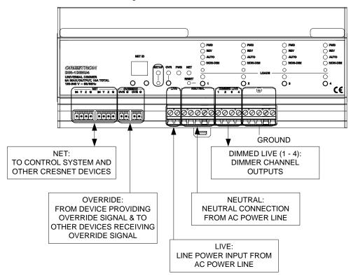
With the circuit breaker turned off, connect the wires to the terminal blocks per the markings provided on the DIN-1DIMU4.
